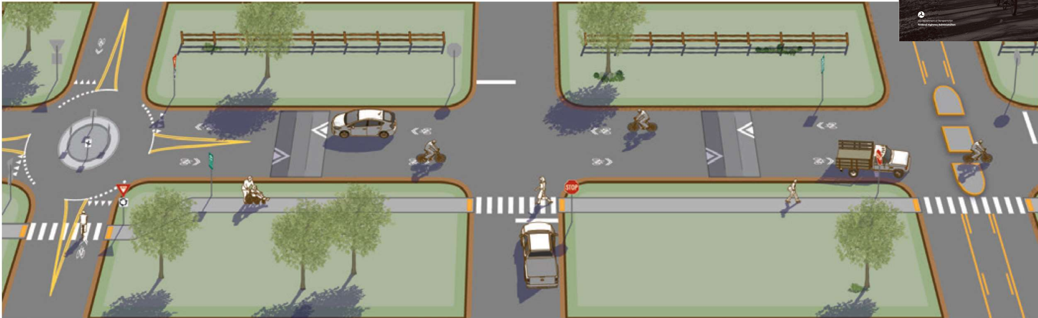
Figure 2-5. Bicycle boulevards combine road markings, traffic-calming measures, and crossing improvements designed to enhance the comfort and priority of bicyclists traveling along the route.
